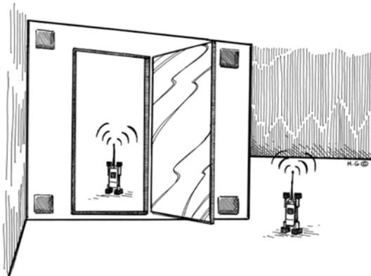
Return to the transmitter and depress the ATTN button. The attenuation will change to 0 dB so that the transmitter output power is now +30 dBm.
