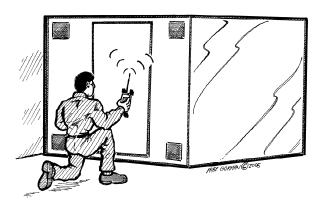
Seam Sniffing in Shield Level Mode
