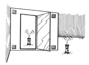
The 60 dB shielding level indication offsets the 60 dB output attenuation on the transmitter. By placing the transmitter and receiver 4-5 feet apart, approximately 30 dB of free space path loss exists. When calibrating the units, the receiver has been designed to account for this amount of path loss in conjunction with the 60 dB of attenuation given by the transmitter. Thus, when the attenuation is removed from the transmitter, the receiver will read very close to 0 dB shield level.
