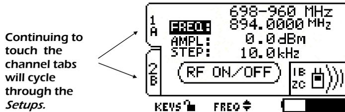
*Setups* for channel 1 can also be changed through the *Channel 1 Setup* Menu, likewise for channel 2.
